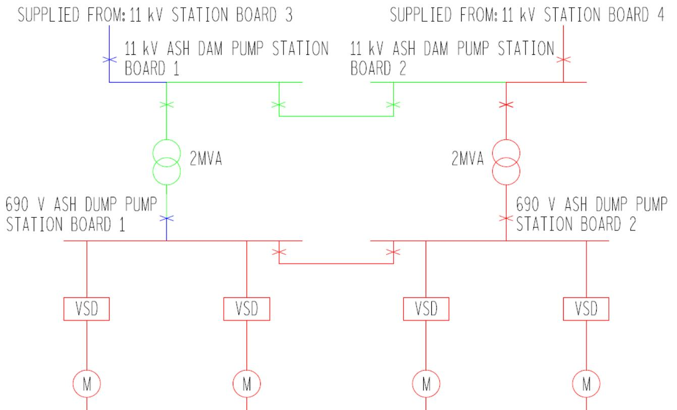
**Figure 5: Schematic of electrical supply network.**
