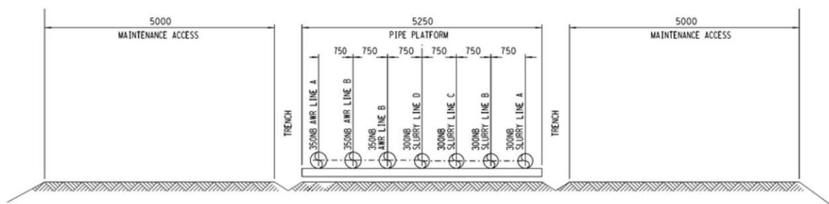
**Figure 3-5: Typical cross section of servitude**
