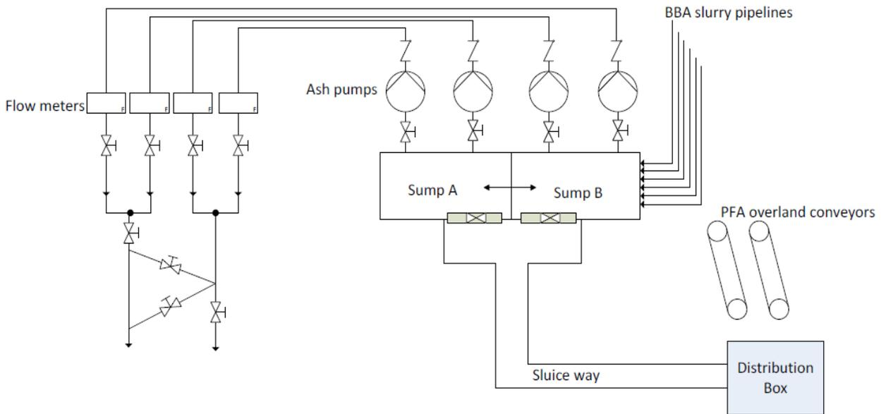
**Figure 1: Kriel Power Station Ash pump house and distribution box layout**
