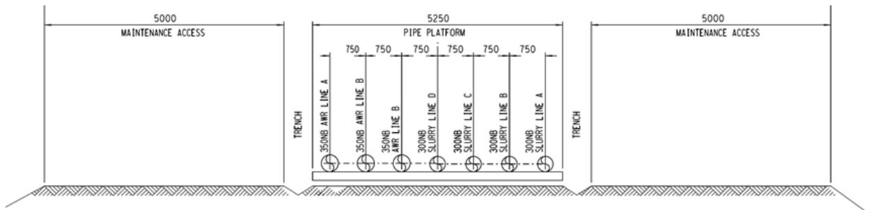
**Figure 8: Typical section through pipeline servitude**
