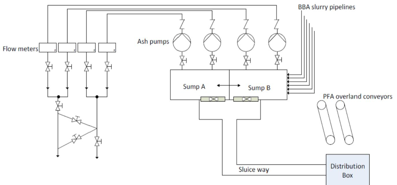
Figure 3-1: KPS ash pump house and distribution box layout
